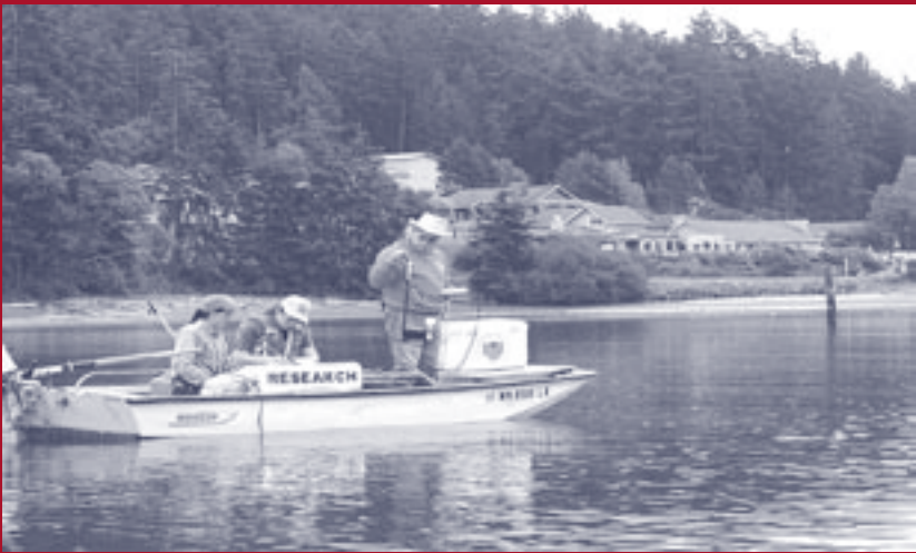
Figure 3. Rebecca, Victoria and Sandy sampling submarine light in the northern reach of Deer Harbor. The instrument Sandy is holding measures light at the surface of the water and through the water as it is lowered to the bottom. Although the sensor is not visible, Rebecca is measuring the temperature and salinity of surface and bottom water. Victoria records data from both sensors.
