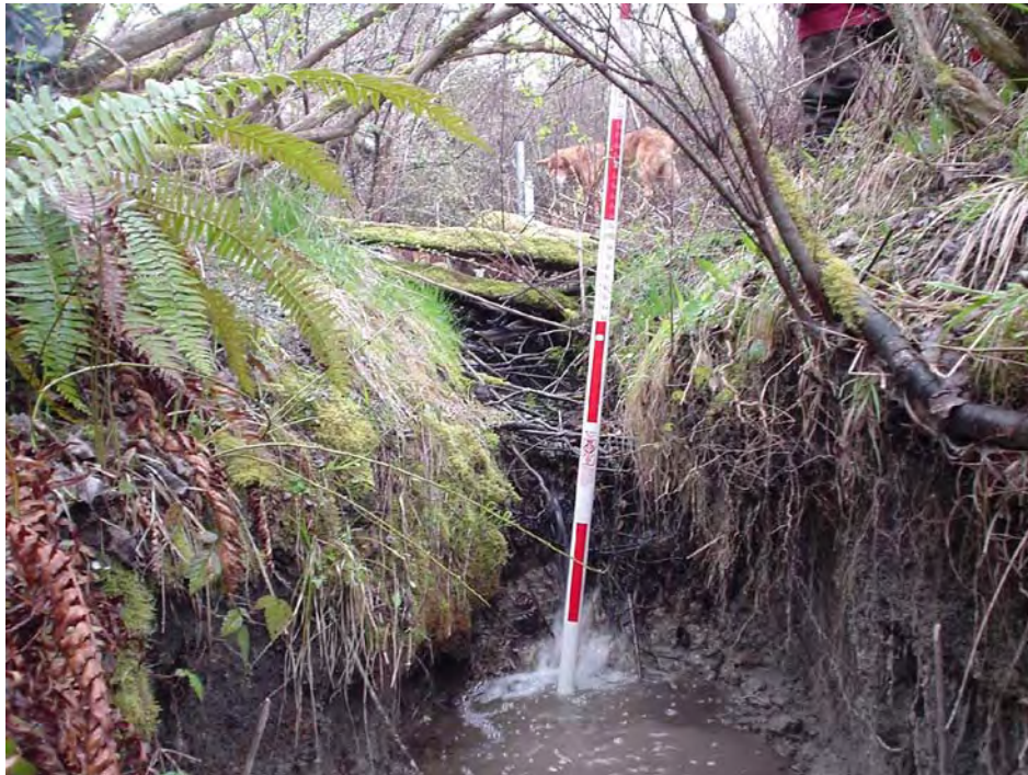
Photo Point A - Photo 1: Headcut channel and clay plunge located at the base of the V-notched weir.
