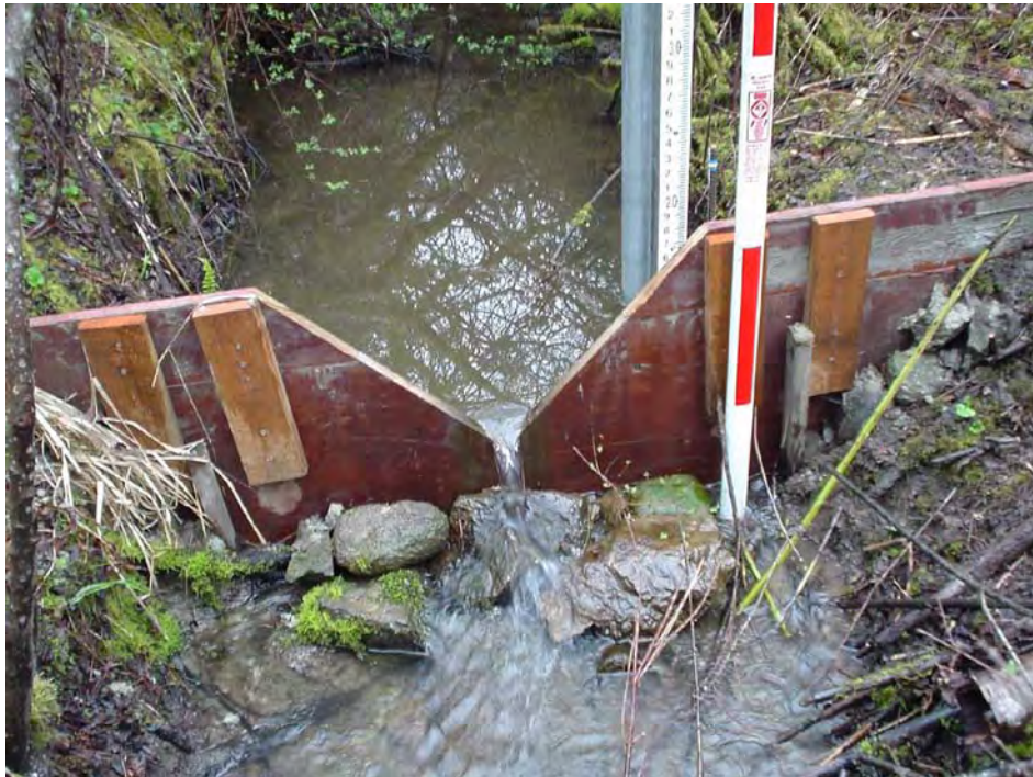
Photo Point A - Photo 2: V-notched plank weir immediately upstream of the headcut in Photo 1. The weir, installed by project partners to evaluate the watershed's hydrograph, exasperates fish passage by increasing the overall drop to the channel below.
